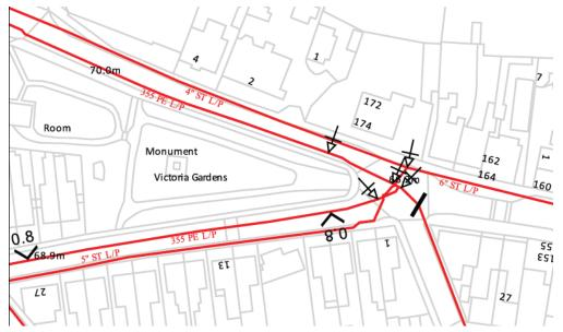
Wales & West Gas services run in the pavement around Western Gateway and cross the road here as well. New planting or resurfacing would need to be cognisant of this and diversion may be required depending on the scope of works proposed.
